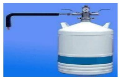
To the right is a liquid nitrogen dispersal system. In use, a dike of insulating foam is made around the IED. The dike is filled with liquid nitrogen which freezes the battery.
