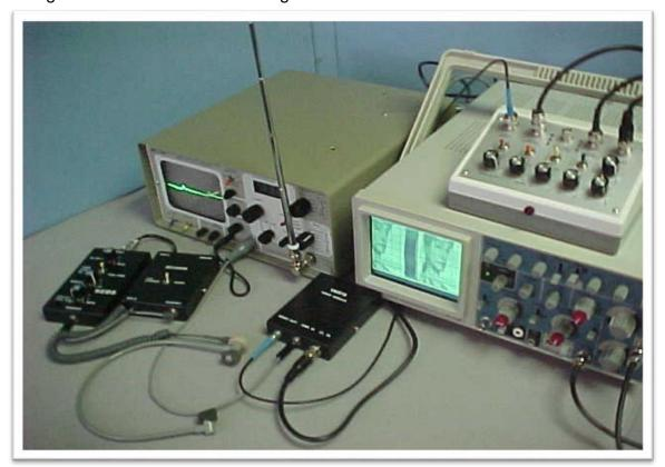
route of the analyzer video and carrier-current demodulator. Center is the VM-515 video demodulator. On top of the oscilloscope is the RAS515 that controls the height, width and intensity of the output signal. The oscilloscope displays the resulting picture. SCD5/SCD-50/SCD-500 low frequency (5 KHz to 700 KHz) carrier current receivers. Detected transmitters on the telephone lines, cable TV, AC power lines or any other wirer pair.
