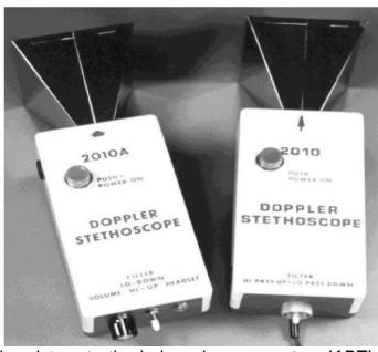
The 2010/2010A Doppler stethoscopes were truly amazing devices. I had accidently discovered the principle behind the homodyne module (transmitter and receiver combined) while working on my Super Man X-ray which I envisioned being able to see inside packages. With them you could hear timers inside sof sided packages such as cardboard boxes,
