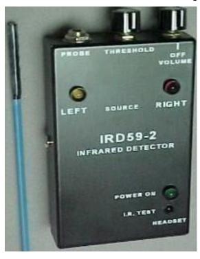
alkaline batteries power the unit. The unit detects the following types of IR beams and reacts as described.
